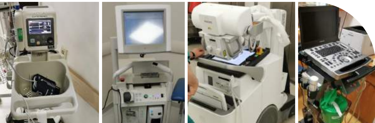
Figures 5-8: Wireless blood pressure, PET-CT, ultrasound and X-Ray devices which require a manual connection to the corporate network upon initial setup or on each usage.
